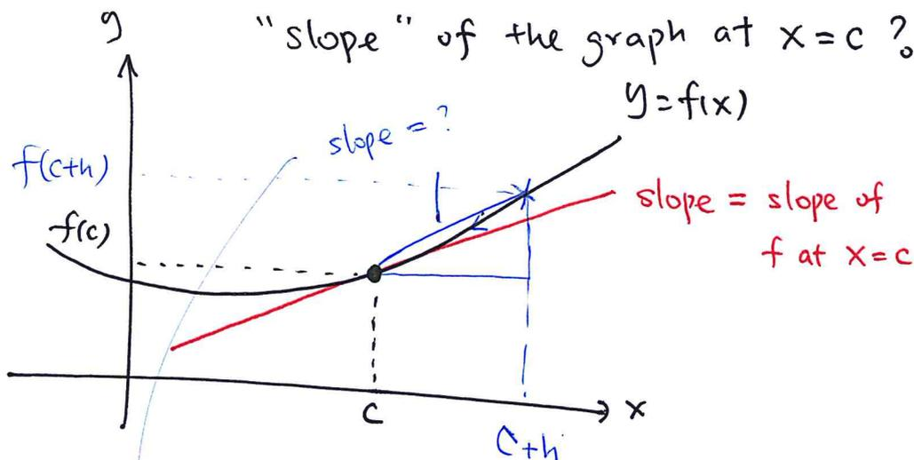
$$\text{Slope} = \frac{f(c+h) - f(c)}{h} =: \left. \frac{\Delta f}{\Delta x} \right|_{x=c} \quad \text{Difference Quotient}$$
